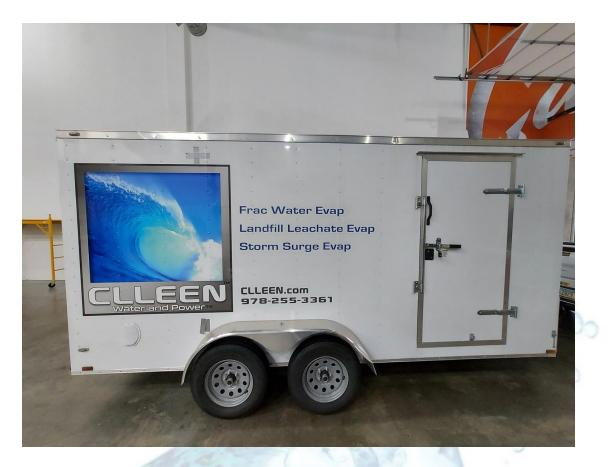
A CLLEEN<sup>™</sup>MOBILE VAP LE 27-foot trailer evaporates 100 gallons per minute of leachate down to dry salts for safe, economical and environmentally friendly re-wasting on the landfill.
