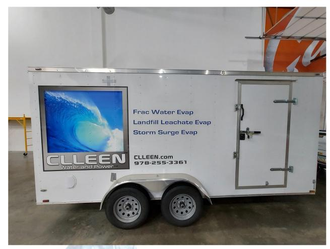
A CLLEEN™MOBILE VAP 16-foot gooseneck trailer evaporates 25 gallons per minute of wastewater down to dry solids for safe, economical transport to a landfill.
